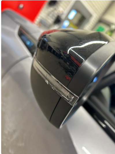
2.1 Krakelering i plast
