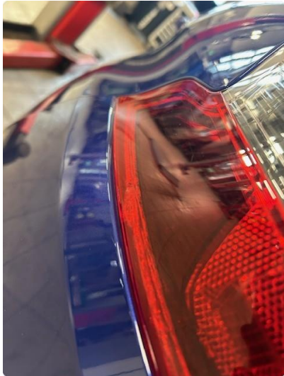
1.1 Krakelering i plast
