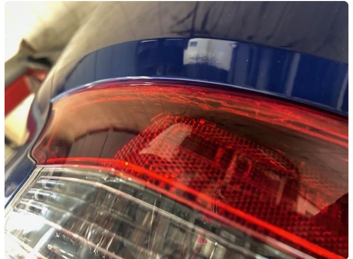
1.1 Krakelering i plast
