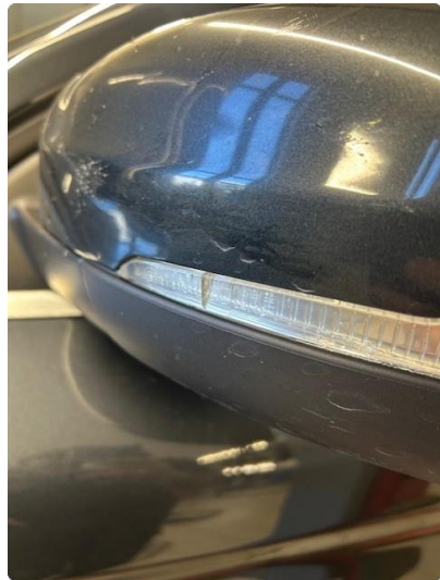
2.1 Krakelering i plast
