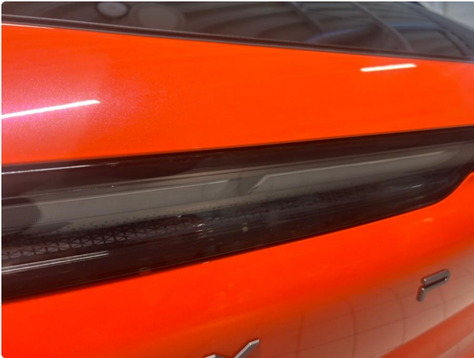
2.1 Krakelering i plast
