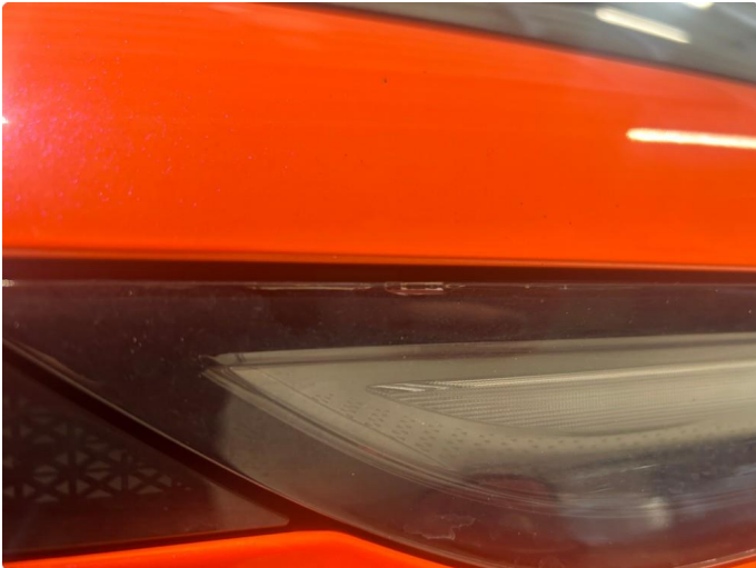
2.1 Krakelering i plast
