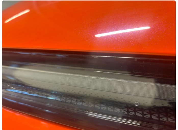
2.1 Krakelering i plast
