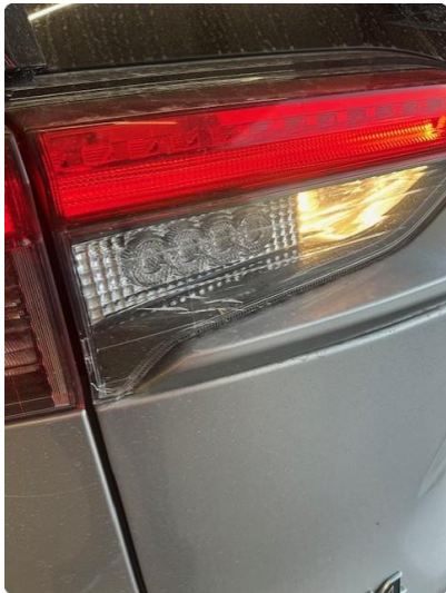
2.1 Krakelering i plast
