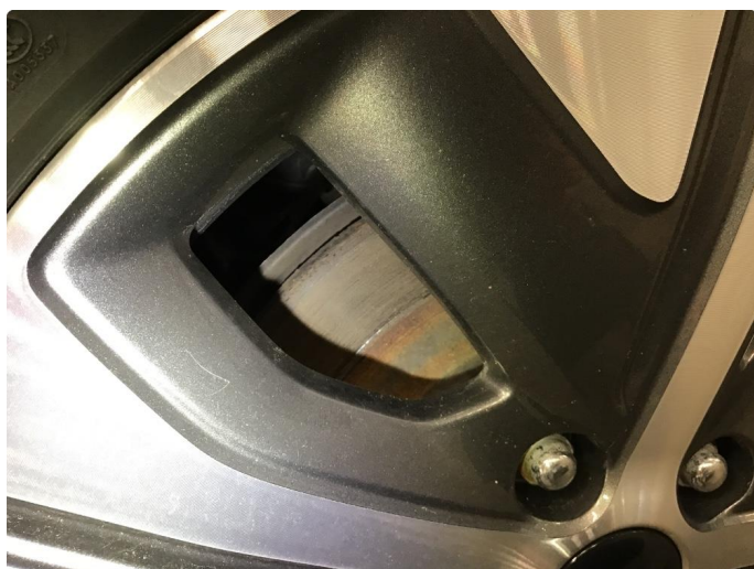
2.1 Mer enn 25% rust
