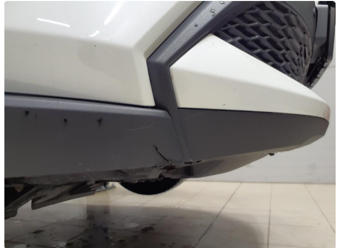
1.2 Liten sprekk underkant
