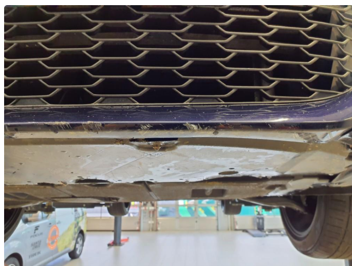
1.2 Noen lakkskader underkant frontfanger
