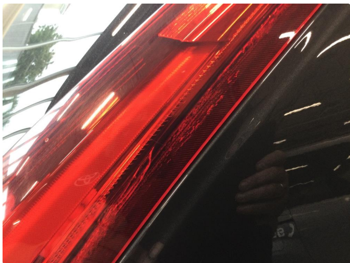
2.1 Krakelering i plast
