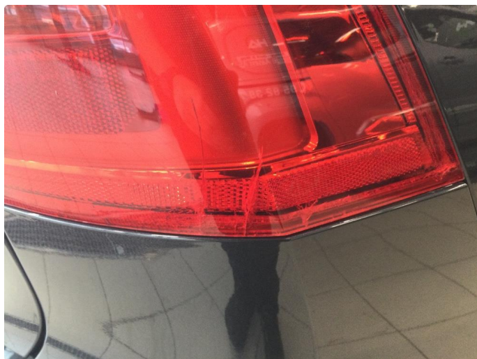
2.1 Krakelering i plast
