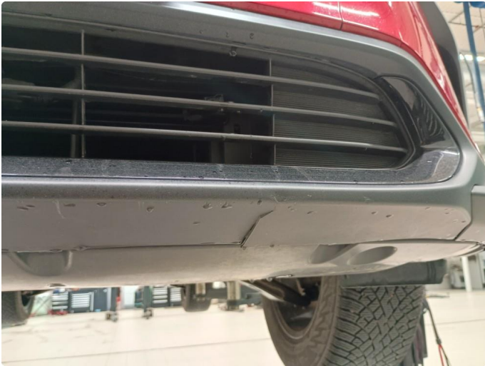
1.3 Liten sprekk underkant frontfanger
