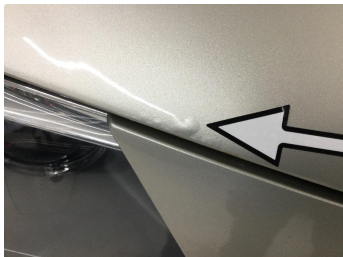
1.2 Rust i fals
