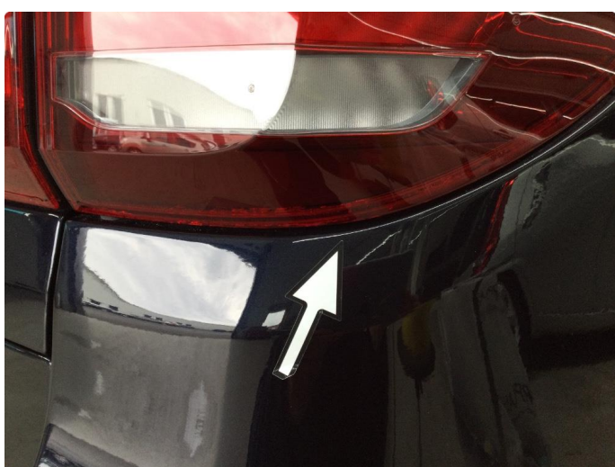
2.1 Krakelering i plast
