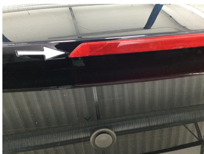
2.2 Krakelering i plast
