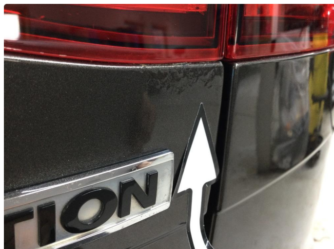
1.2 Rust i fals
