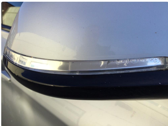
2.2 Krakelering i plast
