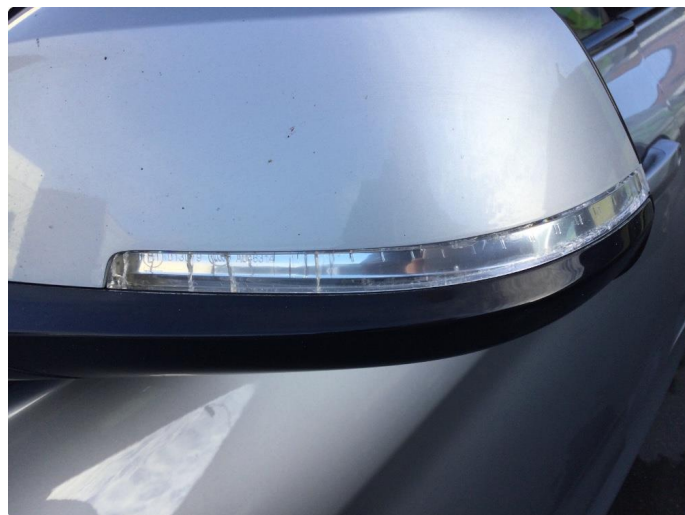
2.2 Krakelering i plast
