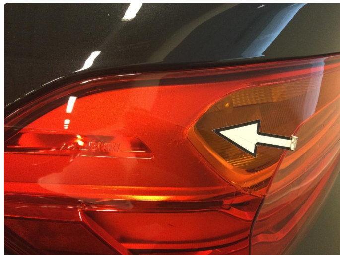
2.1 Krakelering i plast
