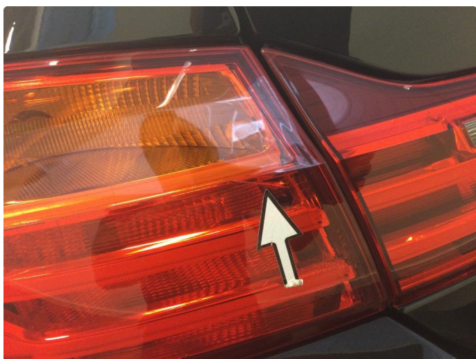
2.1 Krakelering i plast
