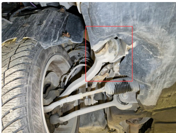
5.3 Utslitt casterforing h+v side fram , sluppet i vulking.
