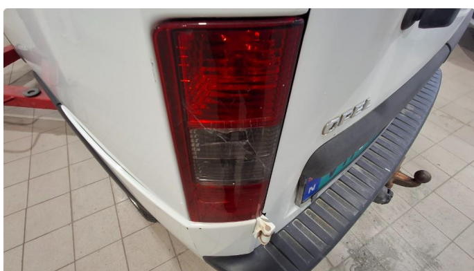
2.2 Defekt / sprukket glass
