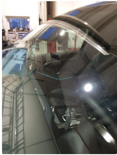
1.4 Steinsprut i synsfelt
