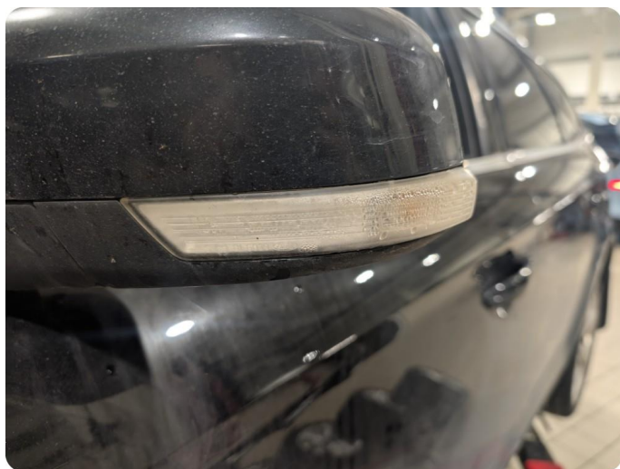
3.4 Vann/dugg Fukt i speilblikers v. side
