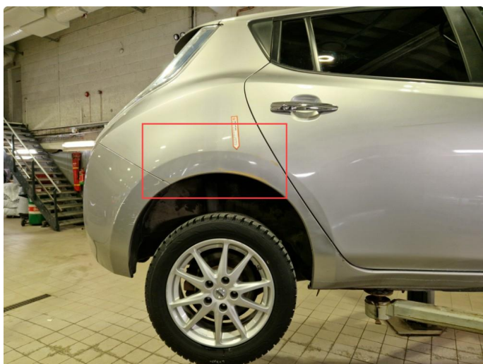
2.8 Rust / bulker / bruksmerker h-bakskjerm.
