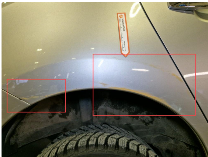
2.8 Rust / bulker / bruksmerker h-bakskjerm.
