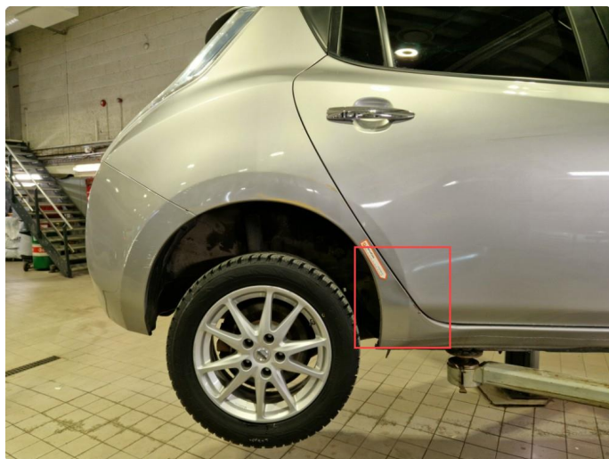
2.8 Rust / bulker / bruksmerker h-bakskjerm.
