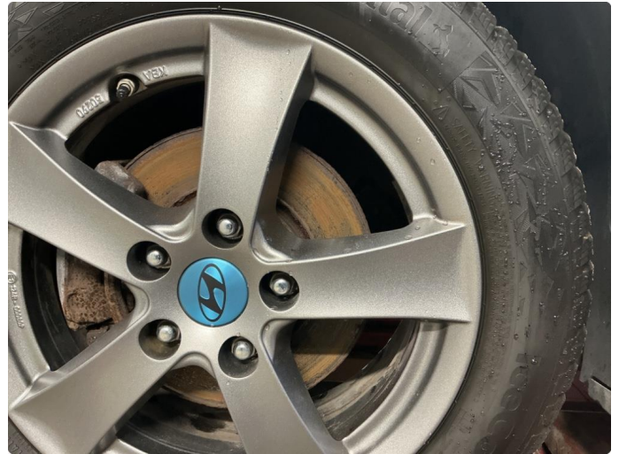
2.1 Mer enn 25% rust
