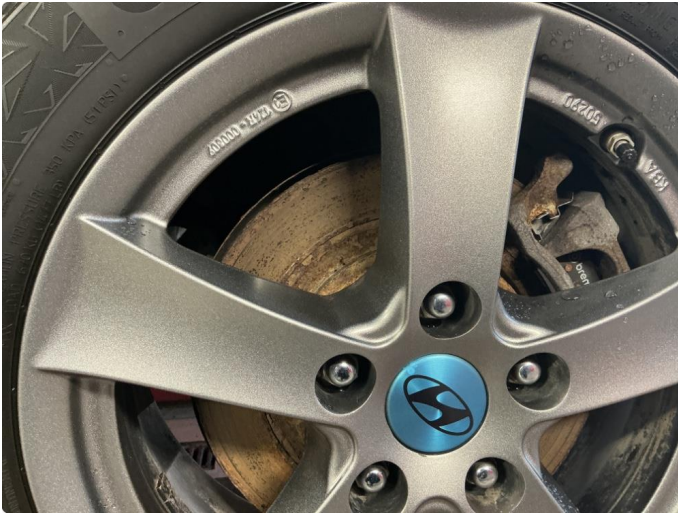
2.1 Mer enn 25% rust
