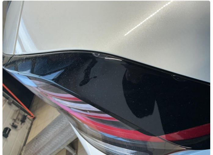
1.1 Krakelering i plast
