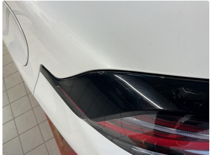
1.1 Krakelering i plast
