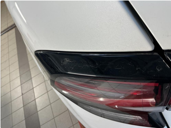
1.1 Krakelering i plast
