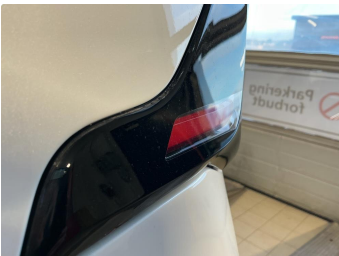
1.1 Krakelering i plast
