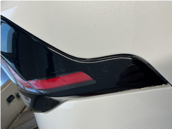
1.1 Krakelering i plast
